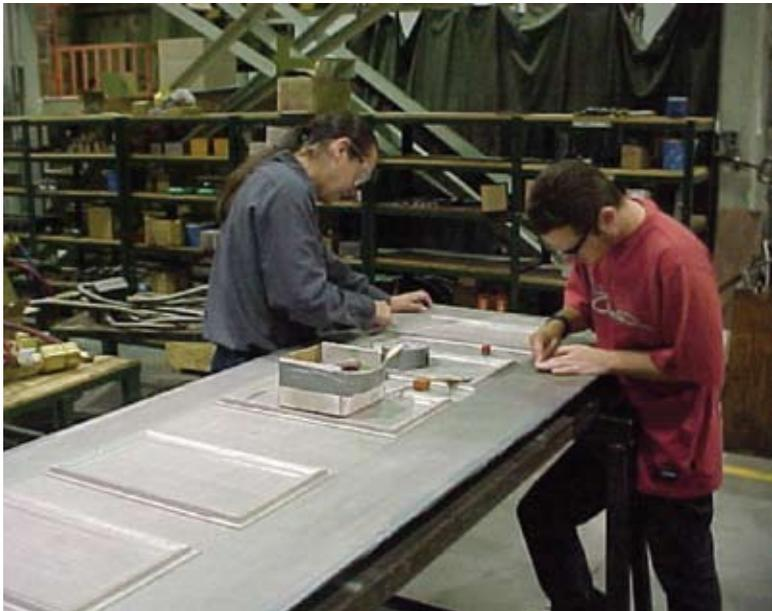
Finished molds require careful handwork to assure true woodgrain details. These molds are used by Weber to press its fiberglass doorskins in an array of styles.
