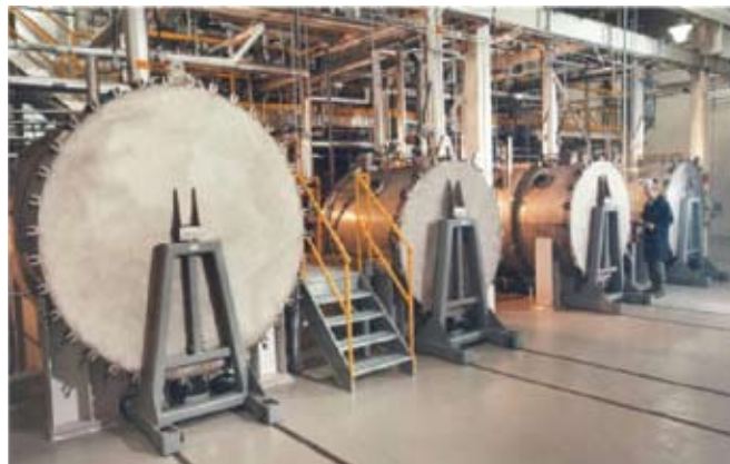
Originally a producer of tooling serving a variety of manufacturing industries, Weber uses a unique nickel vapor deposition process to produce molds that capture fine details.
